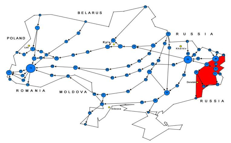
Network analysis shows that nodes 39 and 72 are hubs — the nodes that connect most of the other nodes. These nodes appear to have the highest level of flow betweenness (see Table 1).
